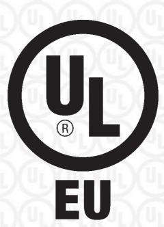
The minimum height of the registered trademark symbol <sup>®</sup> shall be 1 mm. When the overall diameter of the UL-EU Mark is less than 9.5 mm, the trademark symbol may be omitted if it is not legible to the naked eye.
